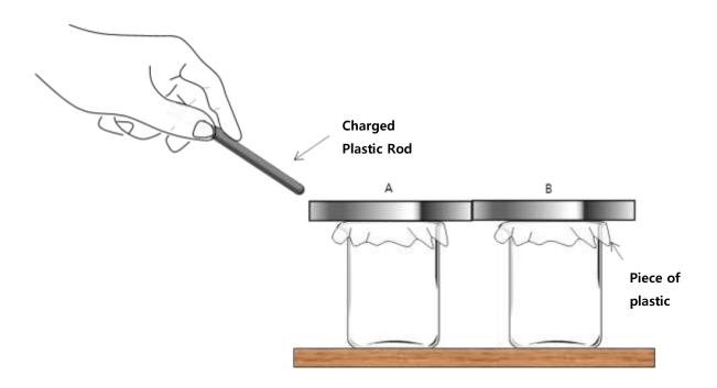
4. While keeping the charged plastic rod close, separate metal rods A and B as shown in the figure.
