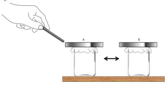
5. Measure the charge values of separated metal rods A and B and the charged plastic rod using the electroscope sensor.
